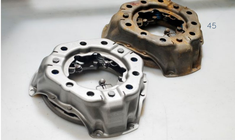
ZF REMAN: Used clutch components are remanufactured and reintegrated into the value chain.
