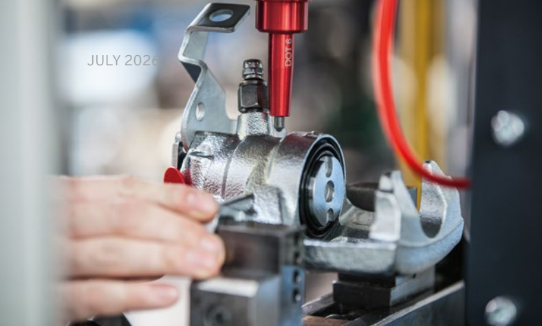
Remanufacturing of brake callipers to enable efficient use of resources in the Automotive Aftermarket.
